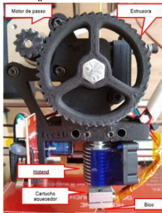
Figura 24 - Extrusora Direct Drive
