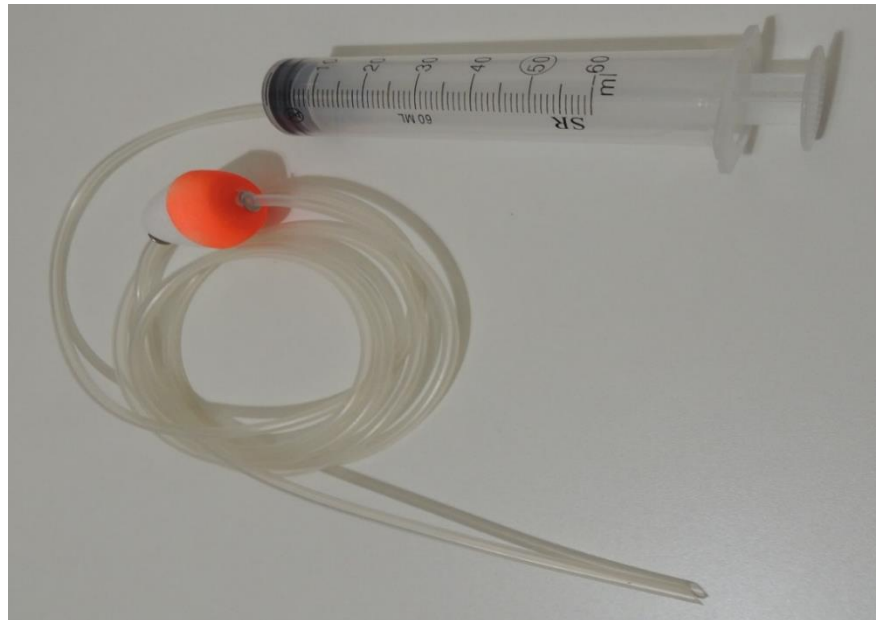
Figure 3 - Water sampling syringe for dissolved oxygen analysis.
