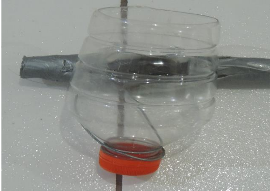
Figure 1 - Water sample collector.
